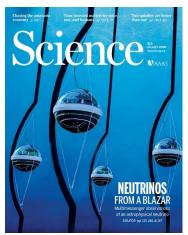
Artist's impression of the IceCube Neutrino Observatory in Antarctica. Spherical digital optical modules (DOMs), each about 35 cm in diameter, are positioned up to 2.5 km deep in the ice. More than 5000 DOMs make up a cubic-kilometre detector weighing more than a billion tons. The DOMs detect the faint flash of light created when a high-energy neutrino interacts with the ice. See pages 115, 146, and 147. Credit: Jamie Yang and Savannah Guthrie/IceCube/NSF
